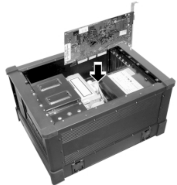
Inserting the add-on card into an open slot.
